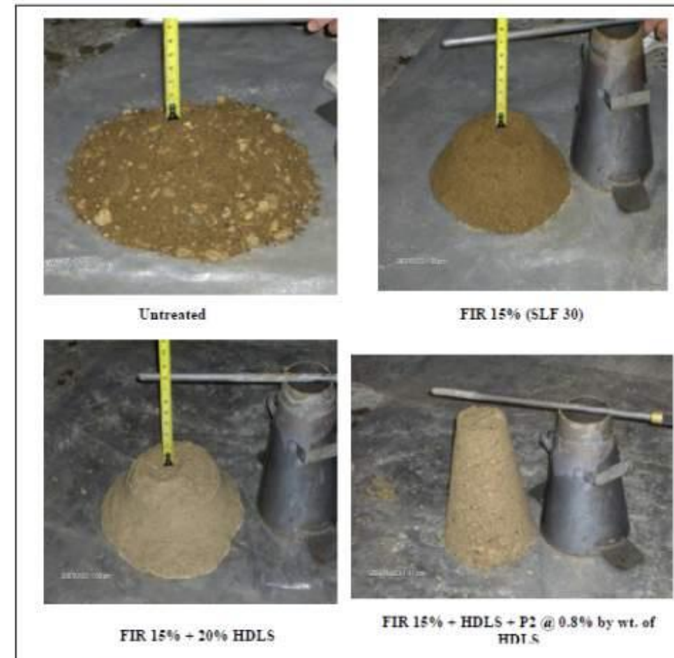
Figure 7 – Photos of soils conditioning on BASF mixture of sand and gravel with low fines
