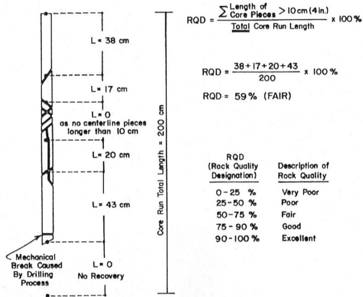
FIG. 1—Procedure for measurement and calculation of RQD.
