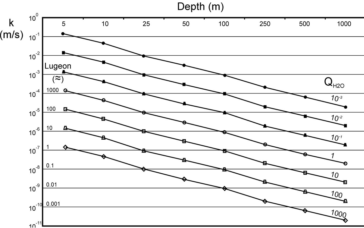
Example of  $Q_{H_2O}$  estimation: Weak, well-jointed rock at 100 m depth with a low assumed joint-wall-compression-strength JCS of 10 MPa:
