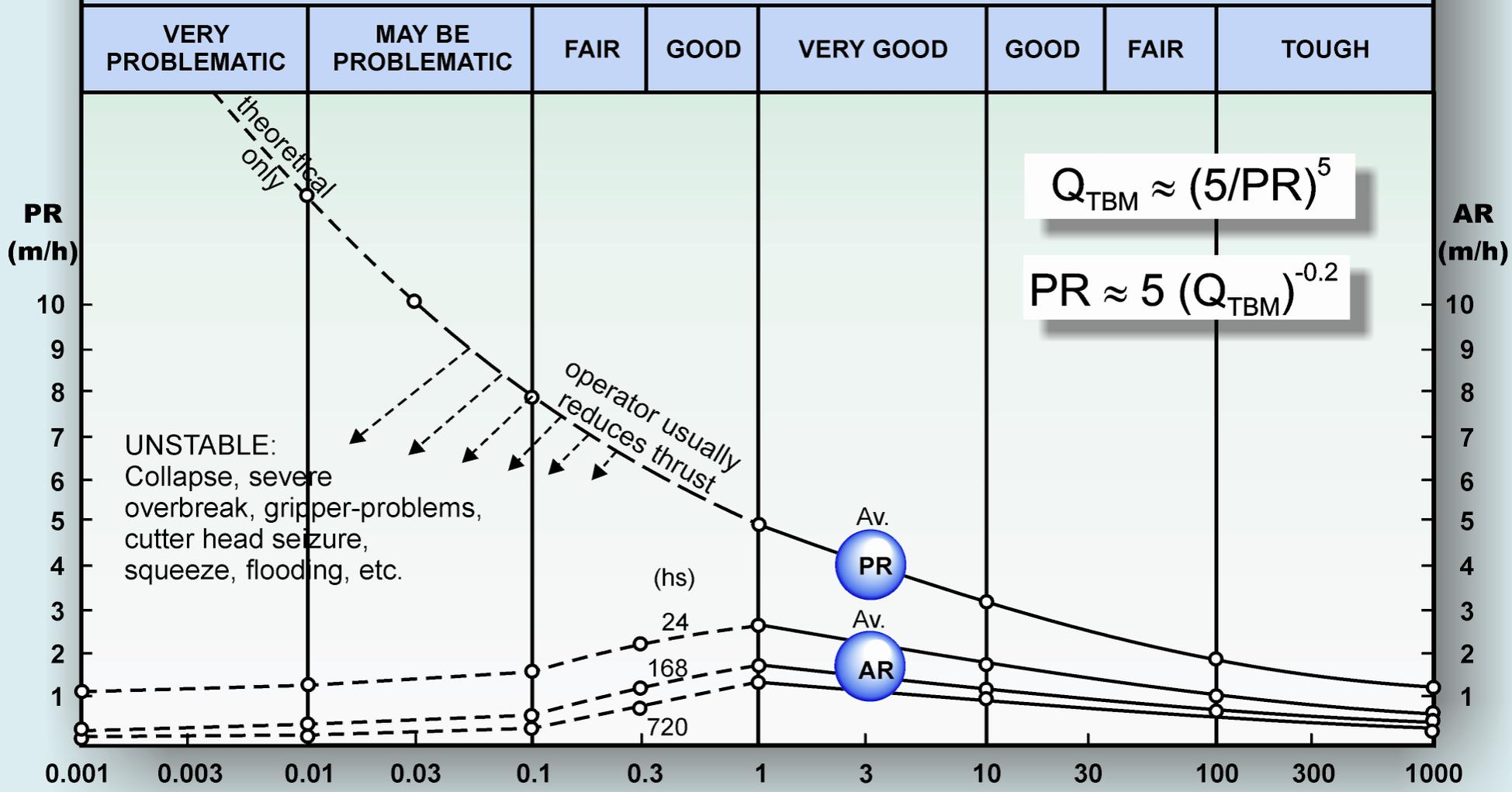
$$Q_{TBM} = \frac{RQD_o}{J_n} \times \frac{J_r}{J_a} \times \frac{J_w}{SRF} \times \frac{SIGMA}{F^{10}/20^9} \times \frac{20}{CLI} \times \frac{q}{20} \times \frac{\sigma_\theta}{5}$$
