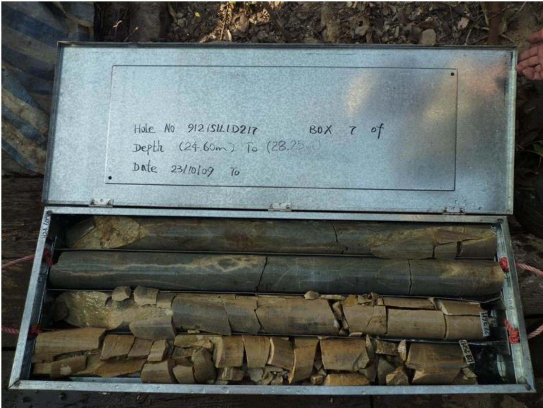
Do not penalise a core because it has a parallel joint causing break-up
